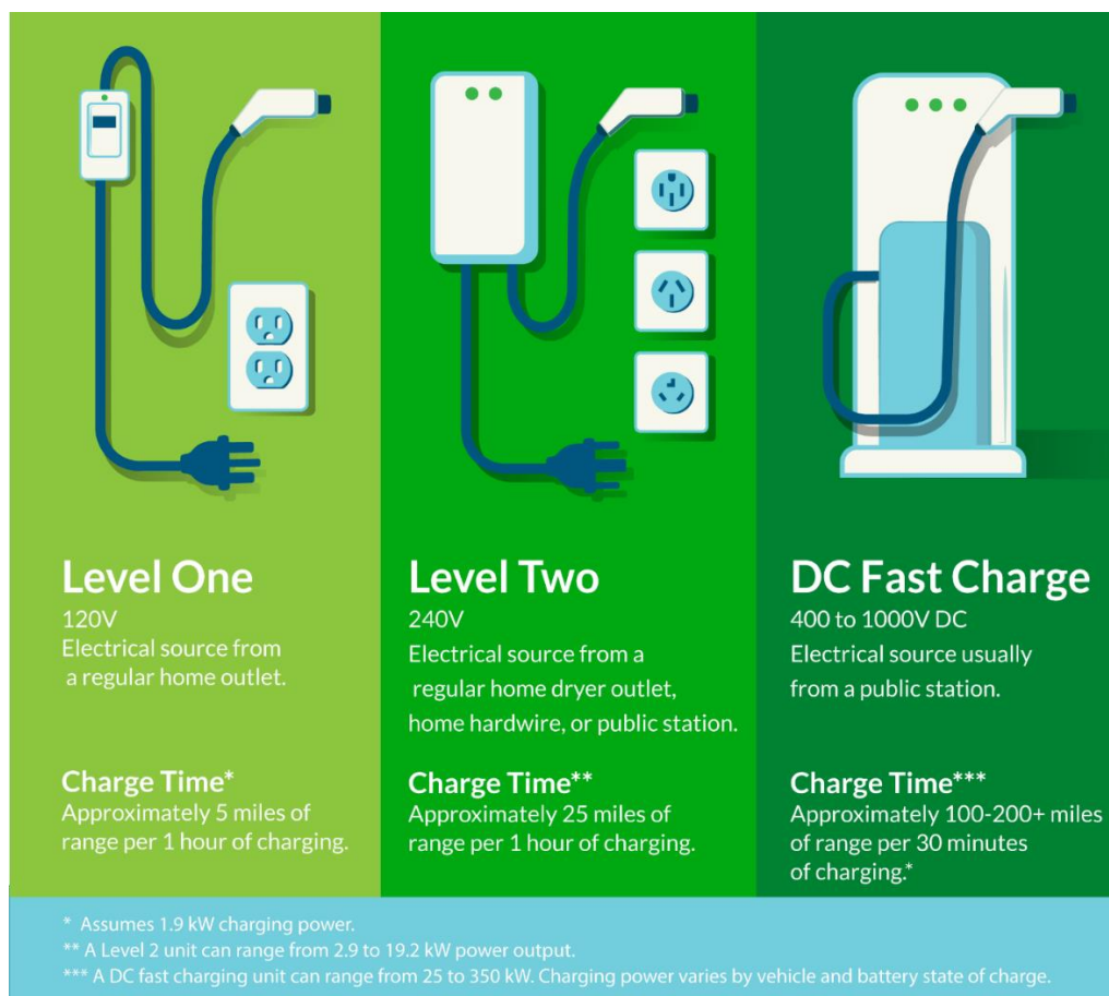
Figure 2: Levels of EV Charging Equipment 23
